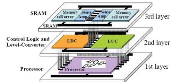
3-D ICs – vertically stacked devices and/or circuit blocks in one circuit. [1, 2]
