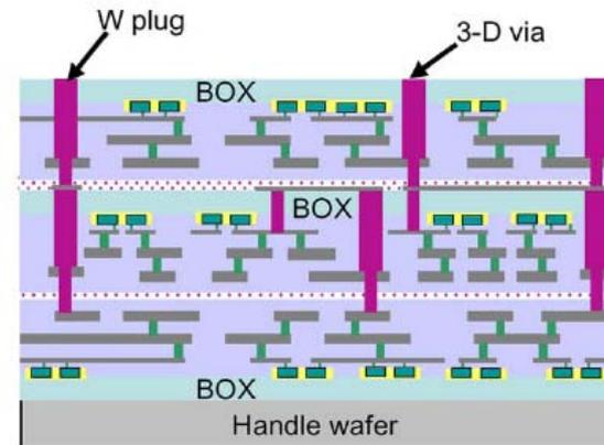
(b) Wafer/die bonding and TSVs [2, 3]
