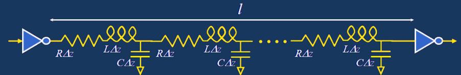
$$C_{line} = Cl \quad R_{line} = Rl \quad L_{line} = Ll$$
