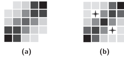
Figure 12: Predicted 2D interconnect density by Lou’s model [23] without (a) and with blockages (b) for a two terminal net. The pins of the net are at the bottom left corner and at the top right corner. Black denotes the highest expected density, white denotes the lowest density.
